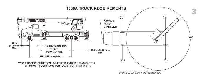
The mounting configuration shown is based on an 85% stability factor. The complete unit must be installed on the truck in accordance with factory requirements, and a test performed to determine actual stability and counterweight requirements, since individual truck chassis vary. If bare truck weights are not met, counterweight will be required. A summary of mounting and truck requirements are:
