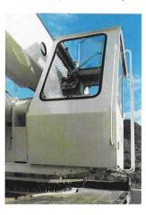
The Lexan top lifts up for ventilation. Other features include a sliding door, front windshield wiper, dome light, circulation fan, optional heater and defroster system, and a cushioned adjustable seat that can be easily positioned for comfort.
