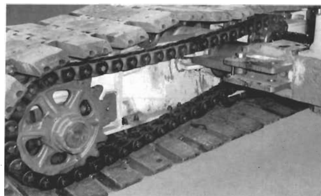
Crawlers at maximum working width with link in position.
