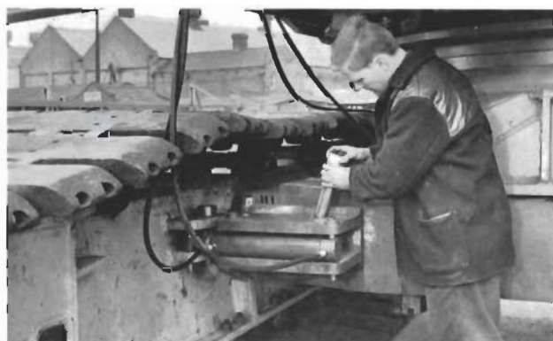
Removing the main pin for widening the crawlers.
