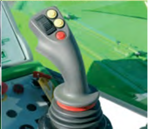
The electro-proportional joystick permits the variation of the boom lifting and extension speed according to the weight of the load being handled.
