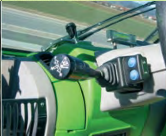
The Finger-Touch forward/reverse control makes it possible for the operator to change driving direction without having to remove his hands from the steering wheel.
