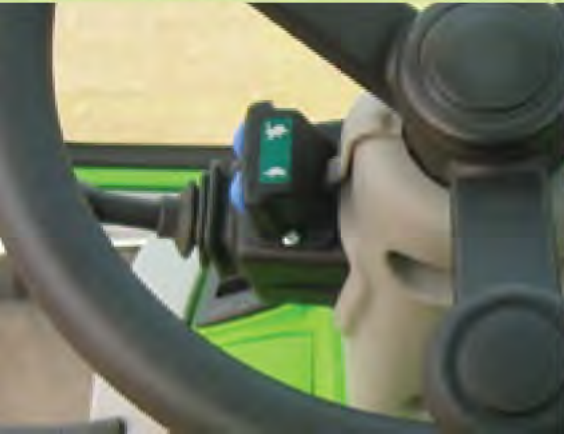
Electrical gear change control with switch conveniently positioned alongside the steering wheel.
