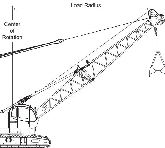
1. Figures represent maximum allowable capacity, and assume level, ground and ideal working conditions.
