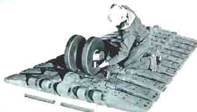
CRAWLER TREADS: 80 inches wide, constructed of cast alloy steel, closed box section design with large center driving lug. 77 treads per crawler side frame. Each pad connected by two high carbon steel pins.
