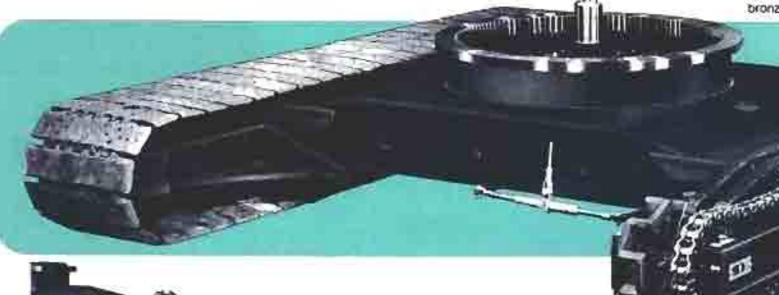
CRAWLER SPROCKET AND TUMBLER: Durable steel casting with flame-hardened teeth and rim. Mounted on stationary shaft supported at both ends by crawler frame for maximum atrength and proper alignment. Sprocket and tumbler revolve on two bronze bushings lubricated by center. grease pocket for efficient operation. Self-cleaning tumbler
