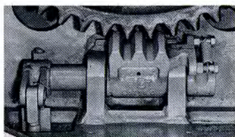
SWING LOCK: Air-operated, spring-loaded, gear-type lock engages swing gear for positive locking.
