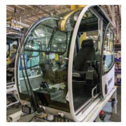
All cabs now come equipped with Heat and AC with 200% more air flow. Adjustable cab tilt speed and crane functions. USB ports for quick software updates or phone charging. More leg space and only one display unit needed for both crane and chassis operations.
