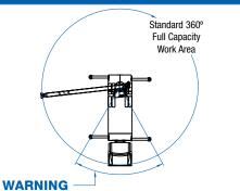
The front tires must be in contact with the ground and the machine level when operating in this area.
