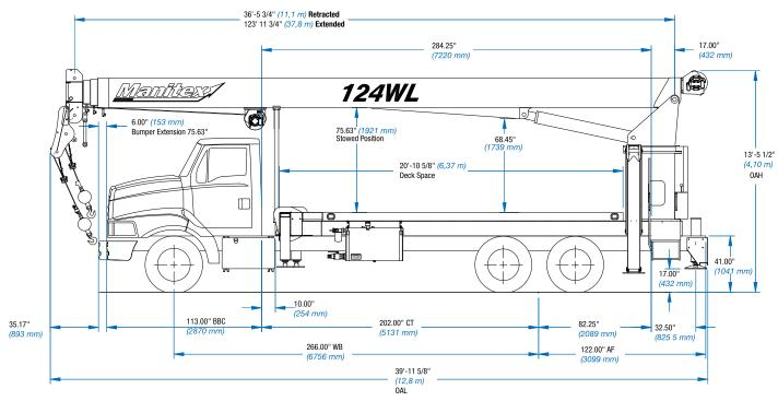
Typical Wireline configuration, does not reflect minimum truck requirement
