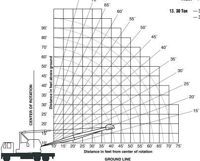
CENTER LINE OF BOOM OVER SIDE NOTE 1 **ON TIRES** OVER REAR CENTER OF ON OUTRIGGERS OUTRIGGERS NOTE 1: These lines determine the limiting position of any load for operation within indicated
