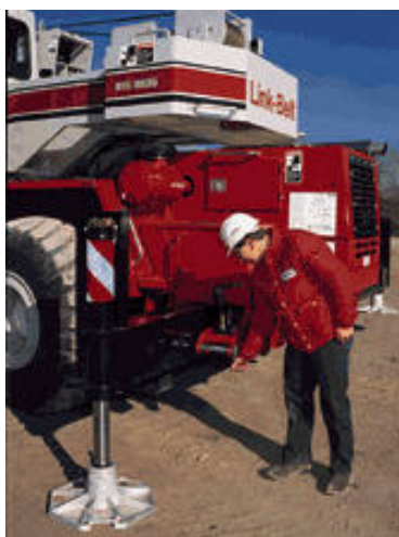
Full Extension Outriggers 20' 6-1/4" (6.25 m) spread
