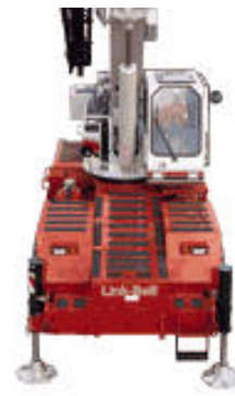
Fully Retracted Outriggers 8' 8-1/4" (2.64 m) spread
