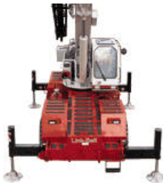
Intermediate Extended Outriggers 14' 8" (4.47 m) spread
