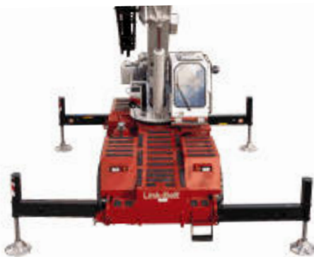
Full Extension Outriggers 20' 6-1/4" (6.25 m) spread
