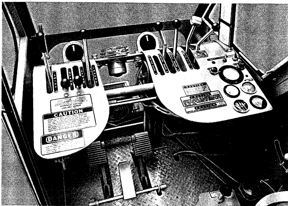
Operator control console
