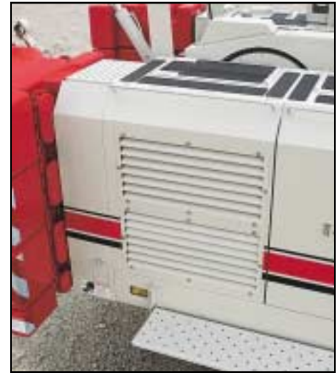
Main hydraulic system has separate cooler, hydraulically-driven fan. Cooler hydraulics — longer lasting, easy to clean (standard)
