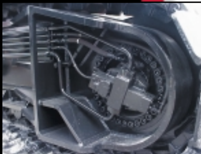
Left: Each treadmember contains a compact travel system that provides independent steering and/or full counter-rotation.
