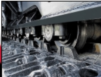
Below: Sealed, oil-filled track rollers, idler and drive planetaries and compact hydrostatic drives add up to outstanding reliability and maintenance-free operation.
