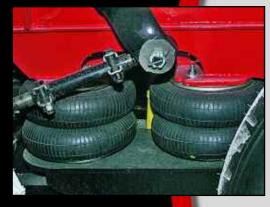
Air-ride suspension front and rear provides a smooth ride and precise handling. Optional air-ride lift system holds the rear suspension retracted while the crane is on outriggers.
