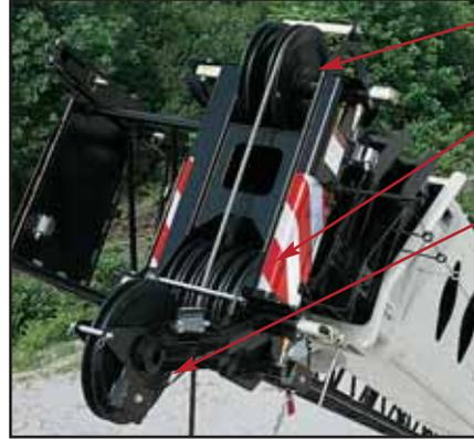
Lightweight nylon head sheaves reduce weight and increase capacity.
