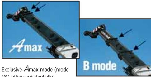
Exclusive **Amax mode** (mode "A") offers substantially increased capacities. **Standard mode** (mode "B") self-proportions all four sections equally.
