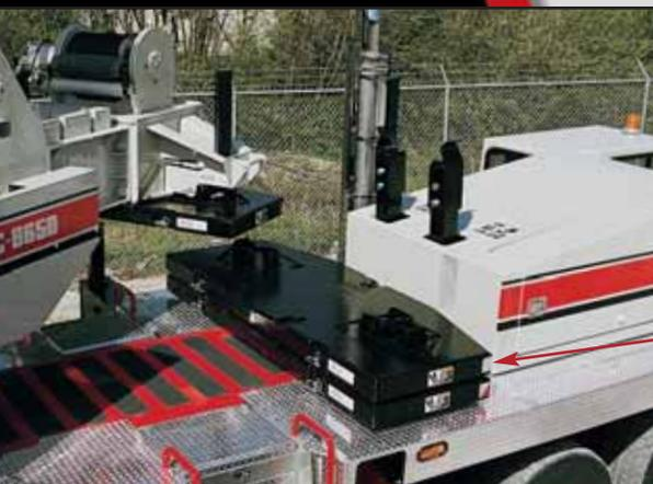
Modular counterweights offer up to four lifting combinations
