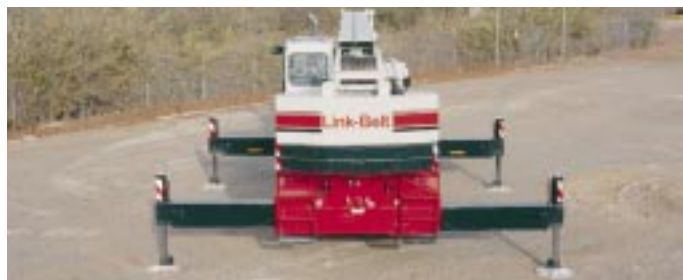
Fully Extended Outriggers 20' 6" (6.25 m) Spread
