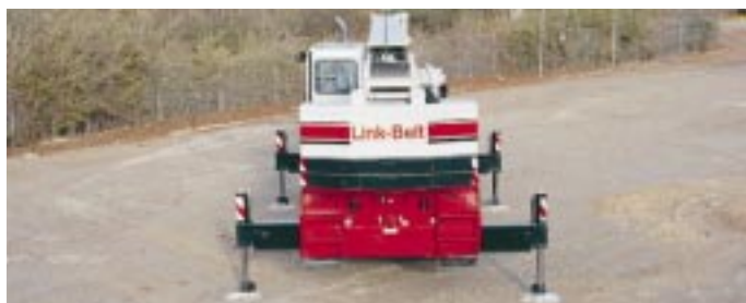
Intermediate Outriggers 14' 2" (4.32 m) Spread
