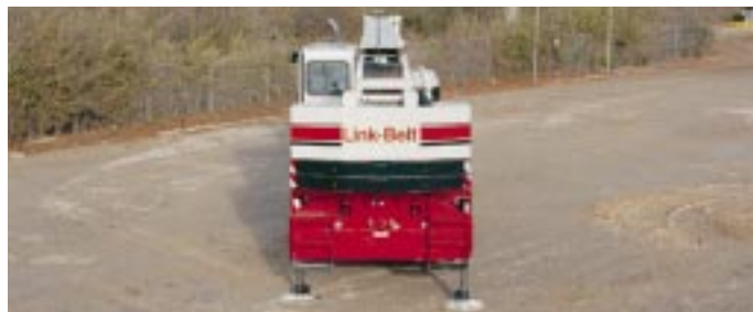
Retracted Outriggers 7' 9" (2.36 m) Spread
