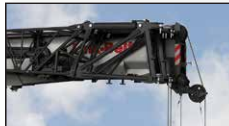
Innovative 12 ft (3.65m) fly is integral to one of the on-board fly options. Over 34 tons (30.8 mt) capacity and one-load two-line lift procedures.
