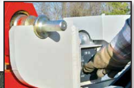
Counterweight removal control station
