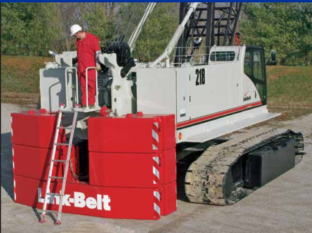
Counterweights lower completely to the ground
