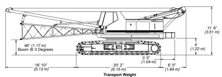
Rope on both drums, Backstops, Catwalks, and 1/3 tank of fuel Tube: 89,751 lbs. (40 710 kg)
