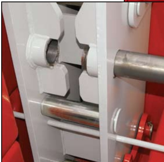
Simple lever action disengages counterweight pins from upper
