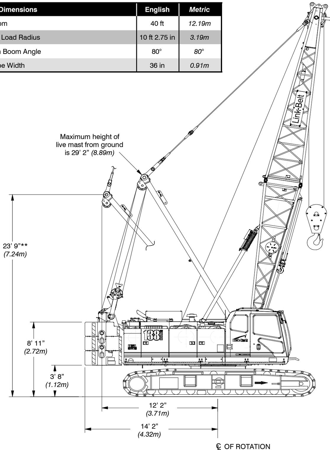
Note: \*\* @ Maximum boom angle (80°) with maximum boom [200 ft (60.96m)], maximum rotation radius occurs.
