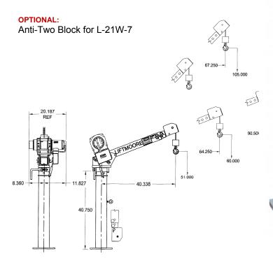
Boom telescopes from 3' 3" to 7' 3"
