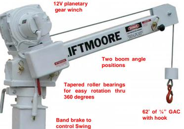
Shown at 20 Degree position and a 3'Load Radius
