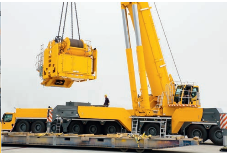
⑥ Self-assembly counterweight frame with drive assembly
