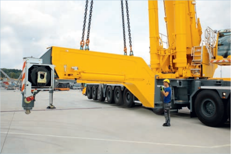
③ Self-assembly of the rear outriggers
