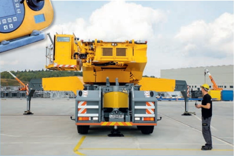
② Additional support at the tail of the vehicle
