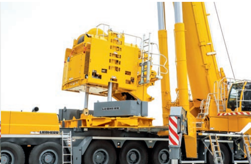
7 Cylinder of the counterweight frame fixed to the ballast ground plate
