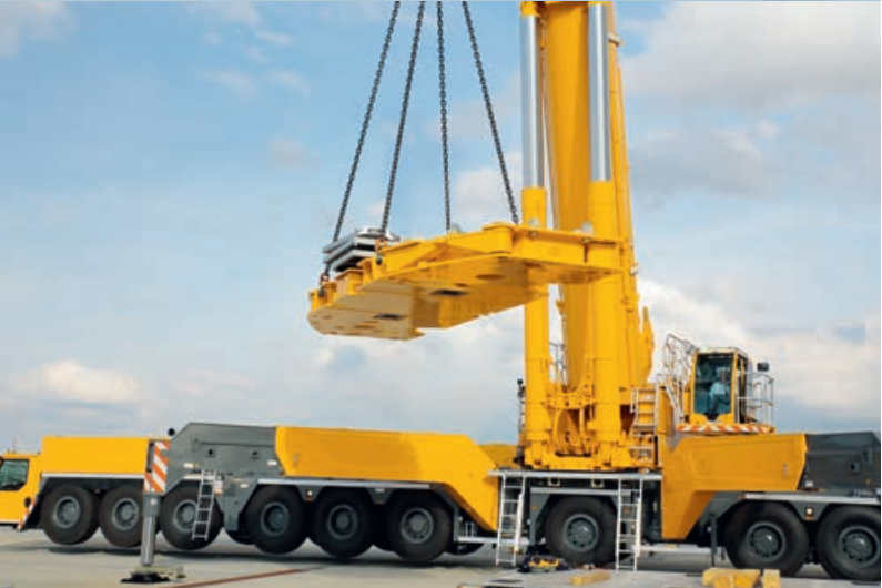
④ Self-assembly counterweight
