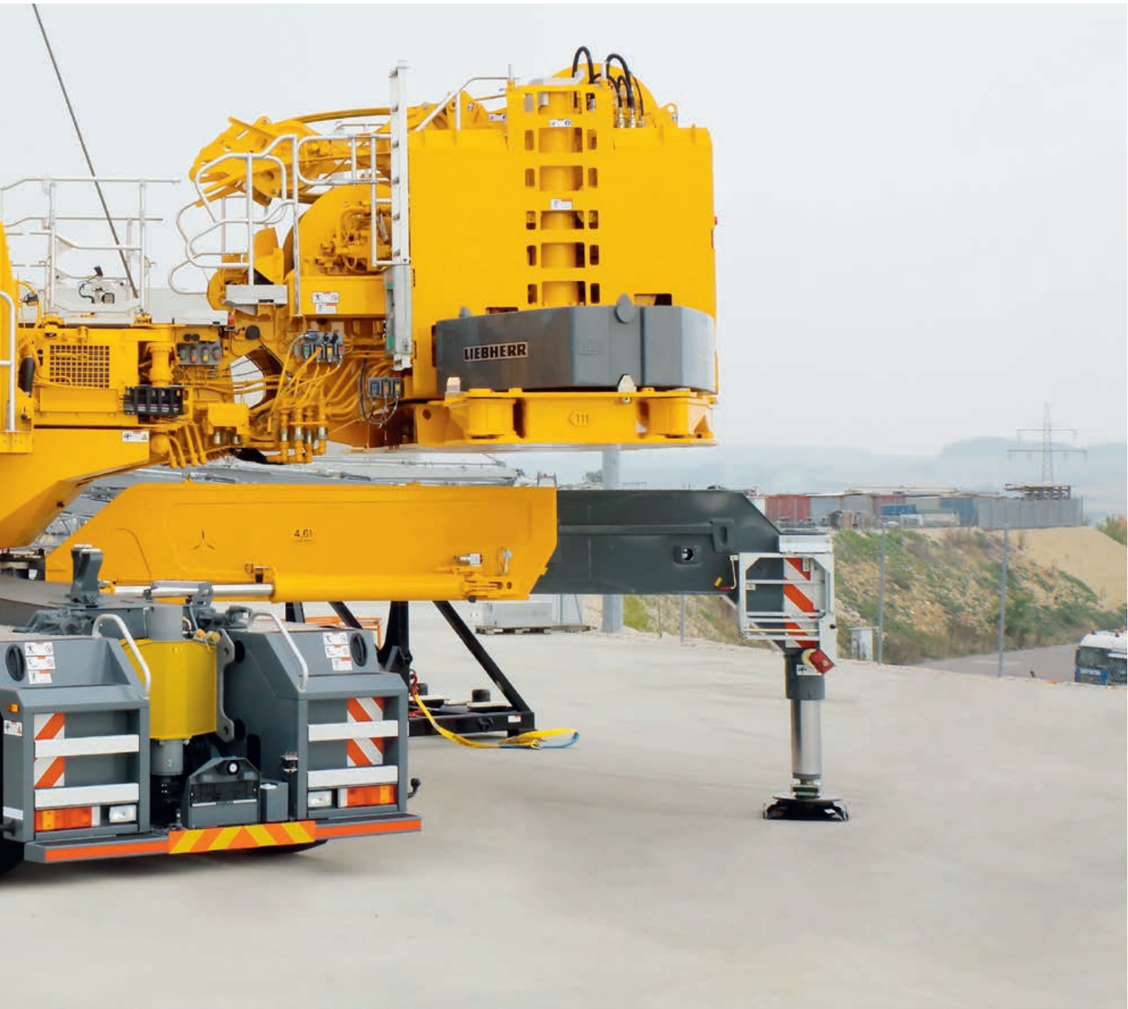
7 Cylinder of the counterweight frame fixed to the ballast ground plate
