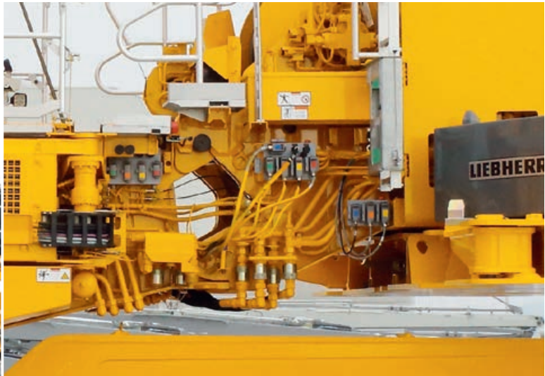
8 Connecting hydraulic and electric quick couplings
