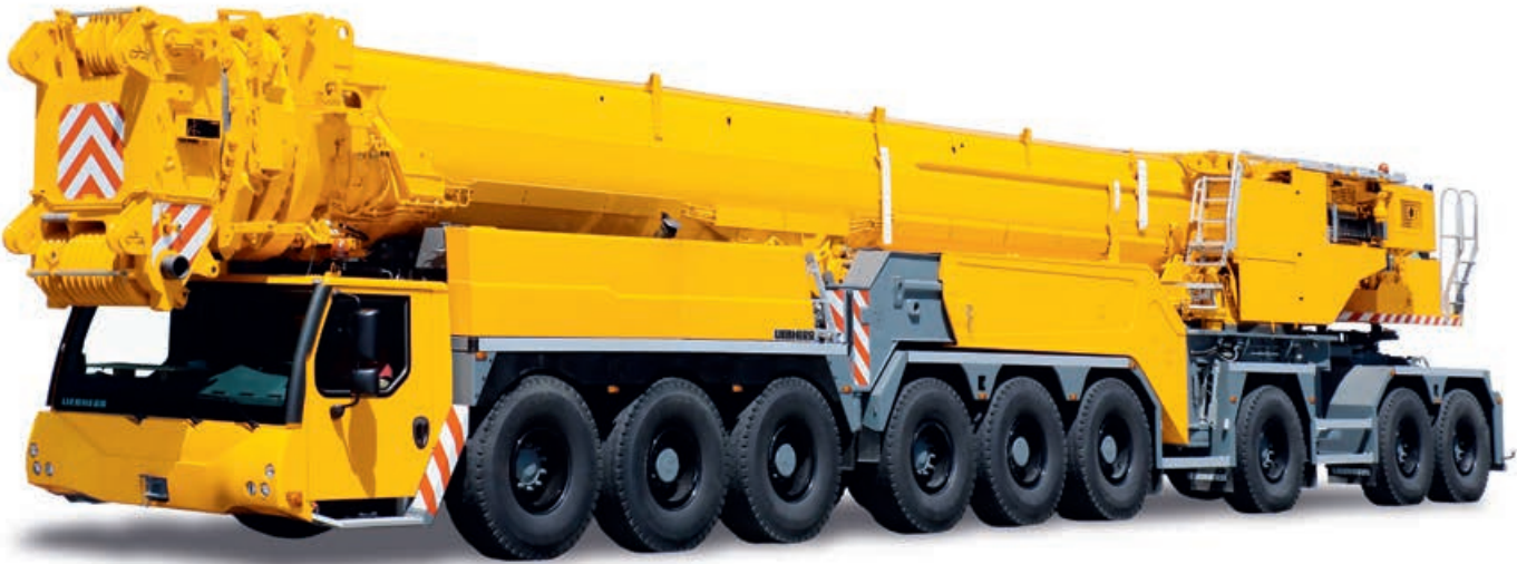
Total weight 108 t at 12 t axle load with front outriggers
