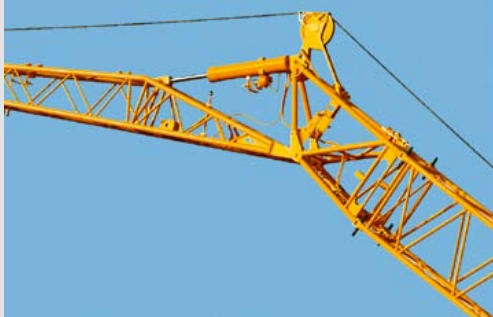
Hydraulically adjustable folding jib (0° to 40°)
