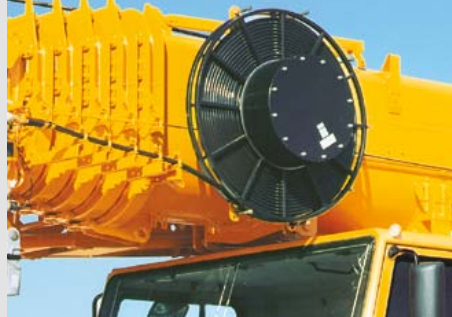
Hose reel for the hydraulic cylinder
