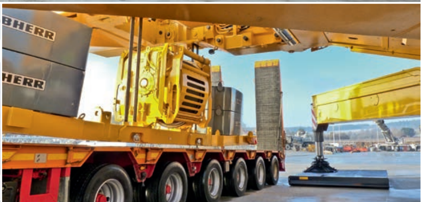
Self assembly of hoist gear 2
