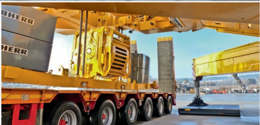
Self assembly of hoist gear 2
