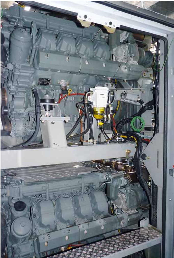
Two complete drive assemblies, Liebherr V8 diesel engines with 500 kW/680 HP each
