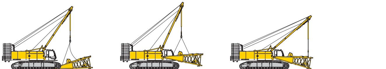
Unloading and assembly of boom foot
