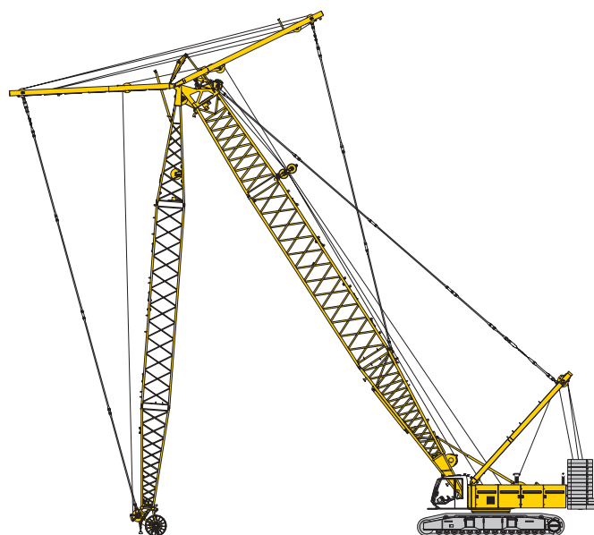
Erecting of main boom and luffing jib
