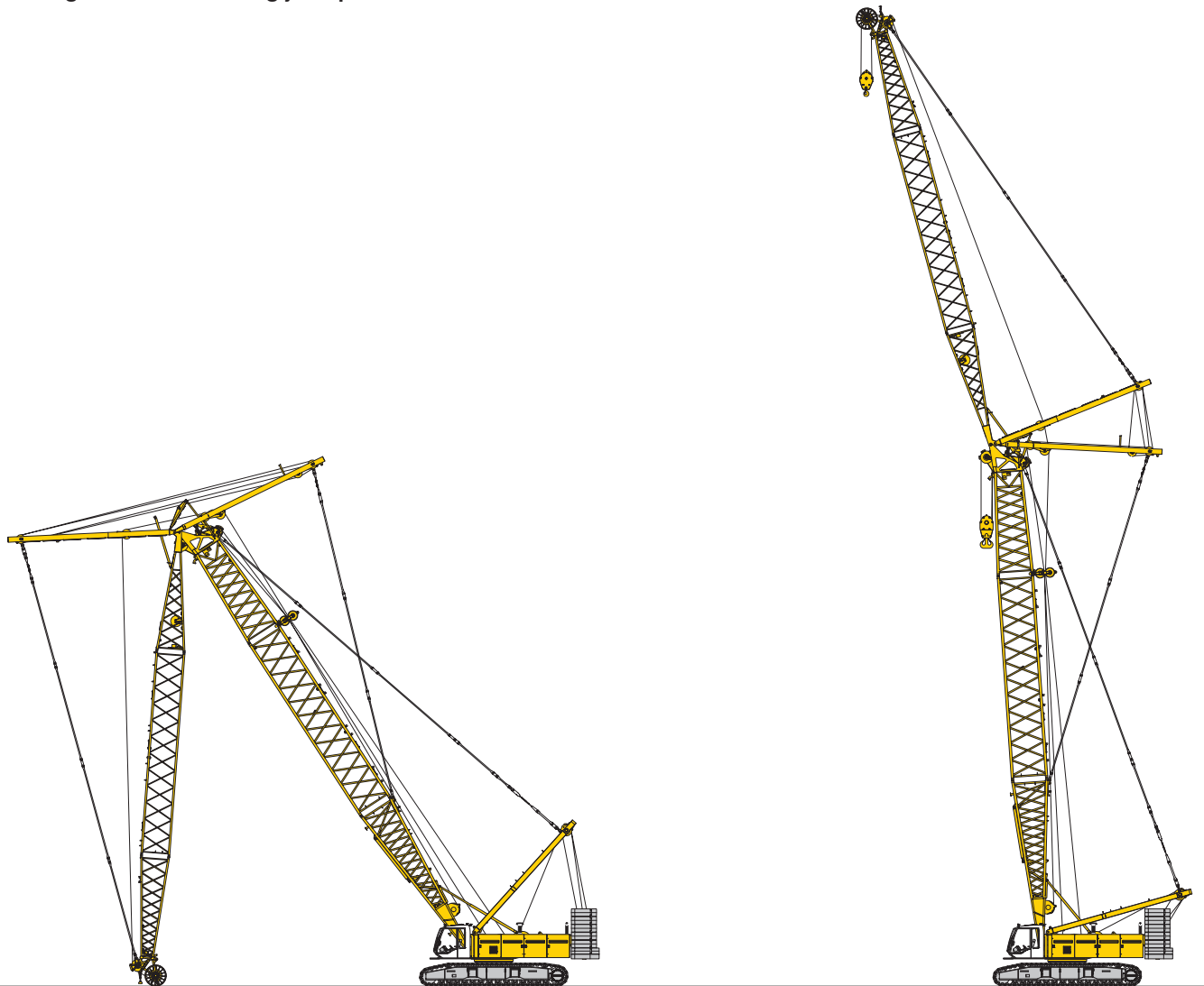
Erecting of main boom and luffing jib
