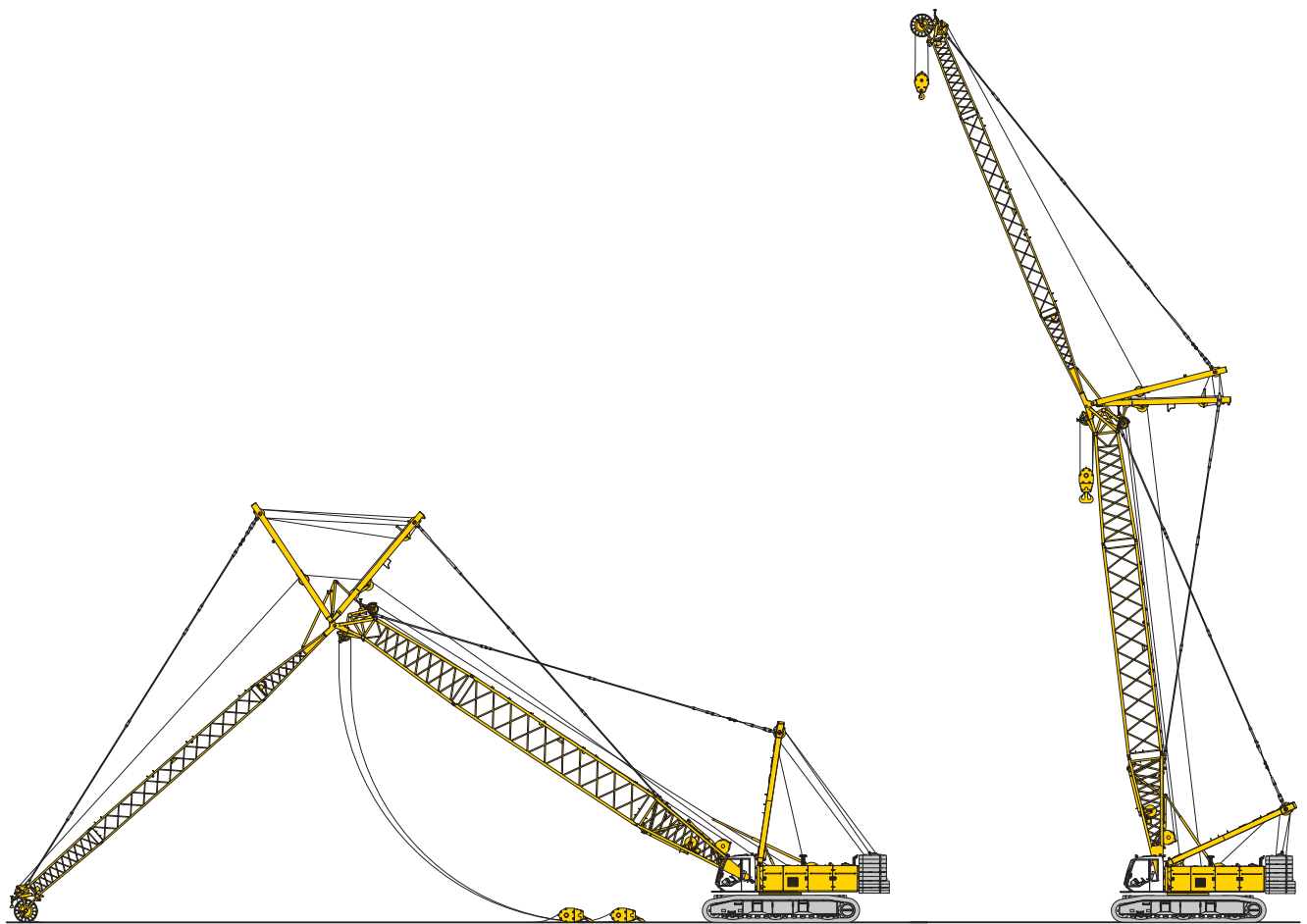
Erecting of main boom and luffing jib
