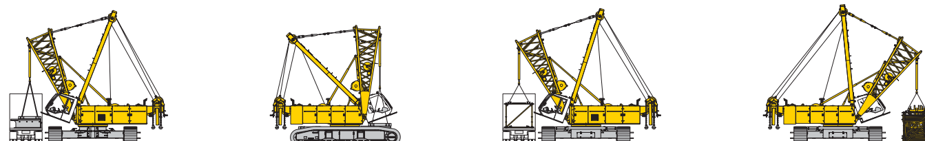
Unloading and assembly of carbody counterweight
