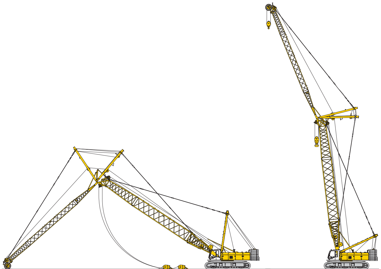
Erecting of main boom and luffing jib
