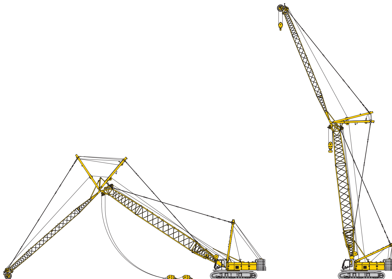
Erecting of main boom and luffing jib
