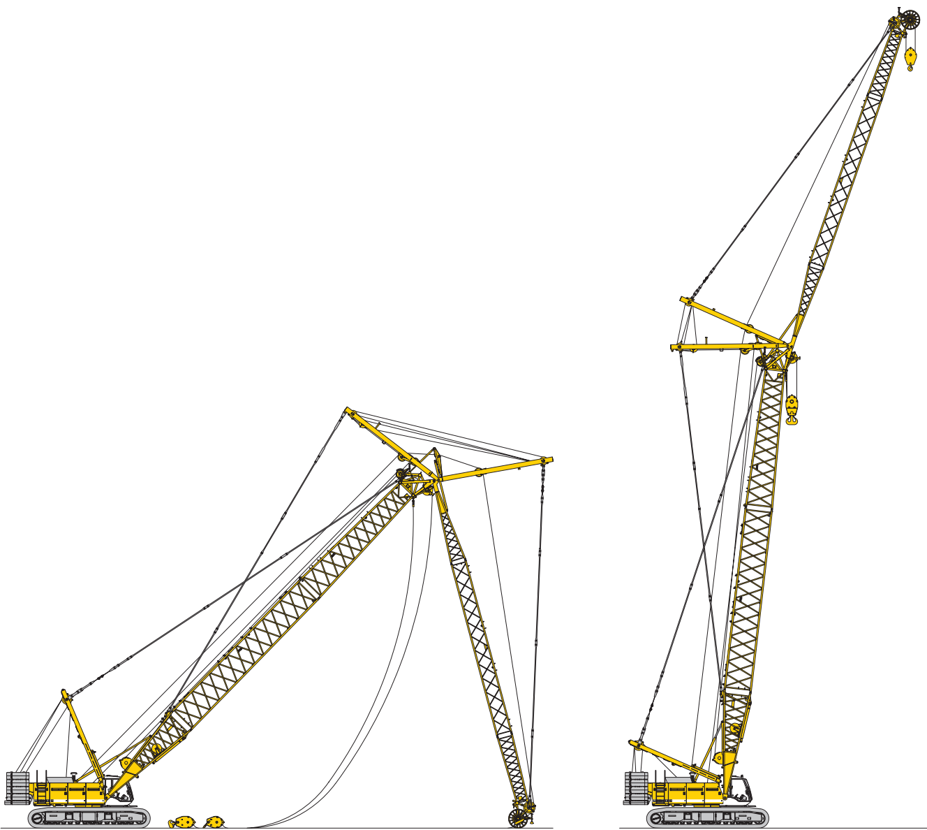
Erecting of main boom and luffing jib
