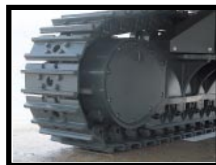
Sturdy guards shield the travel motors against damage from rocks.
