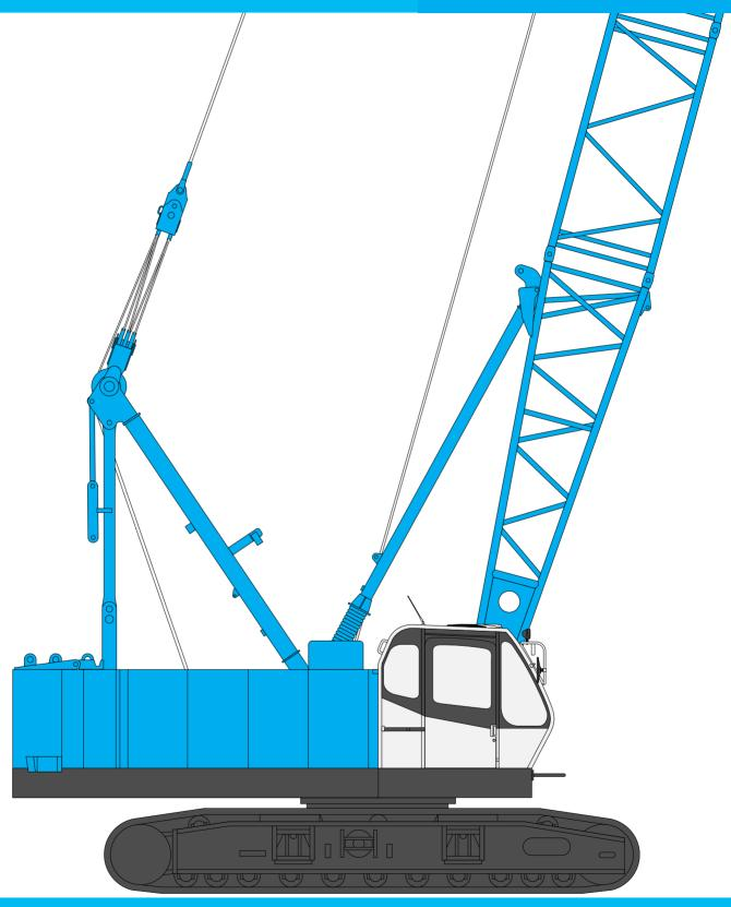
Max. Lifting Capacity: 90 t x 3.4 m\*
