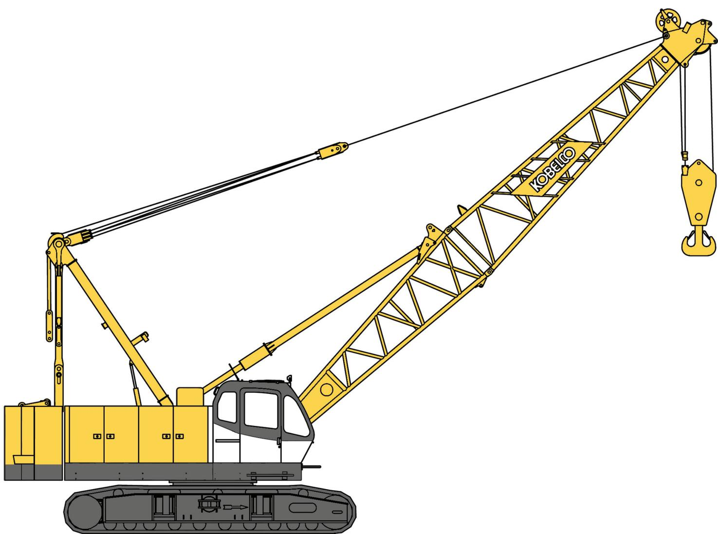
**Max. Lift Capacity: 85 US Tons**
