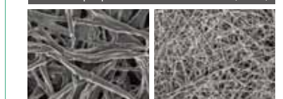
Conventional filter (paper fiber) Super-fine filter (glass fiber)
