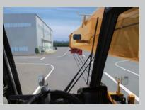
Making front view wider and assuring more safety at travelling with lower position of boom foot pin and smaller front overhang
