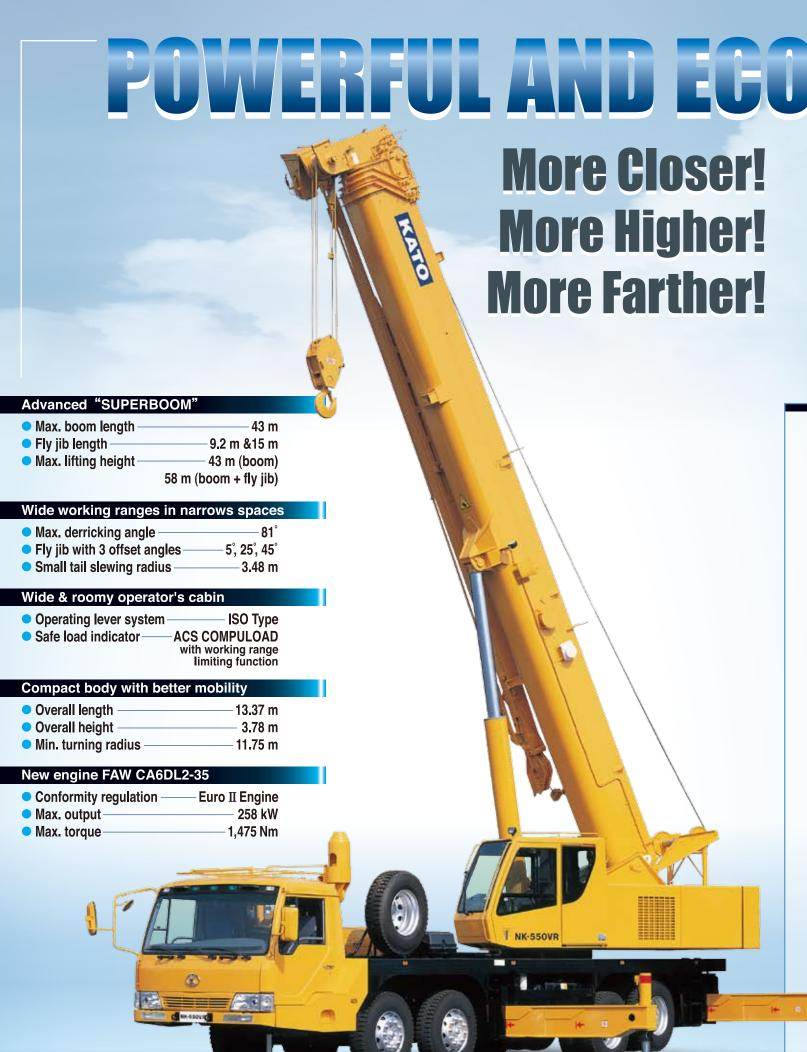
Solid 43m SUPERBOOM combined with 15m fly jib offers you steady operation and wider working ranges in narrow spaces.
