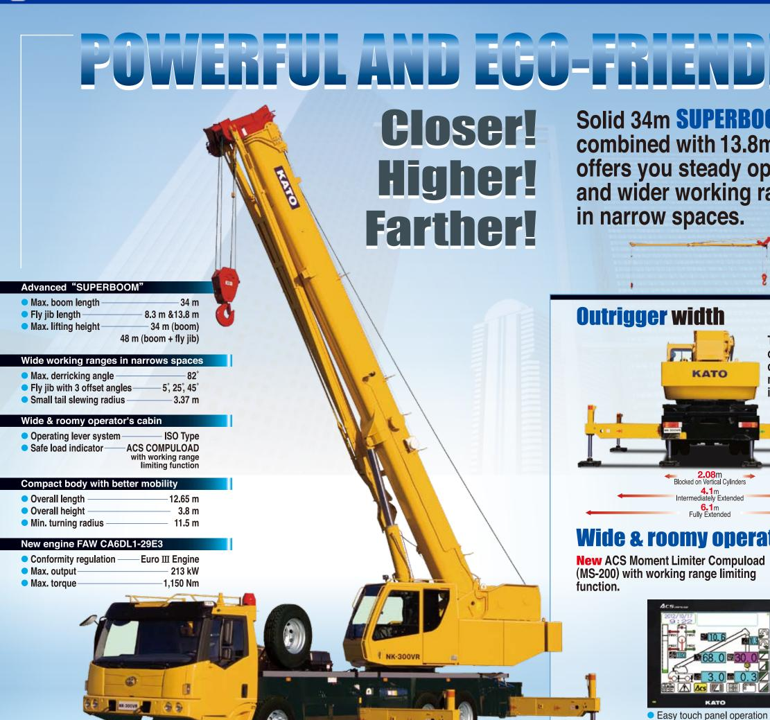
Solid 34m SUPERBOOM combined with 13.8m fly jib offers you steady operation and wider working ranges
