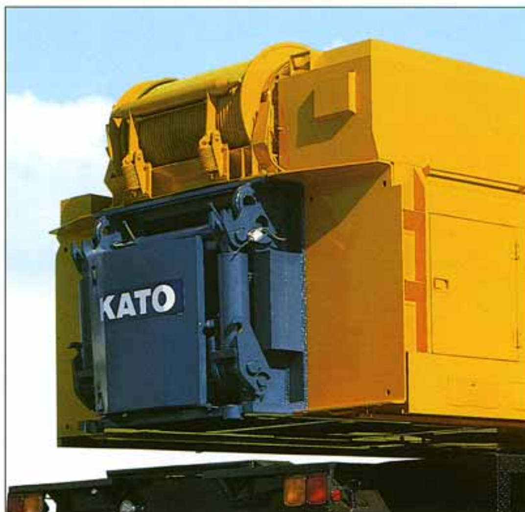
Linkage-type counterweight removal device
