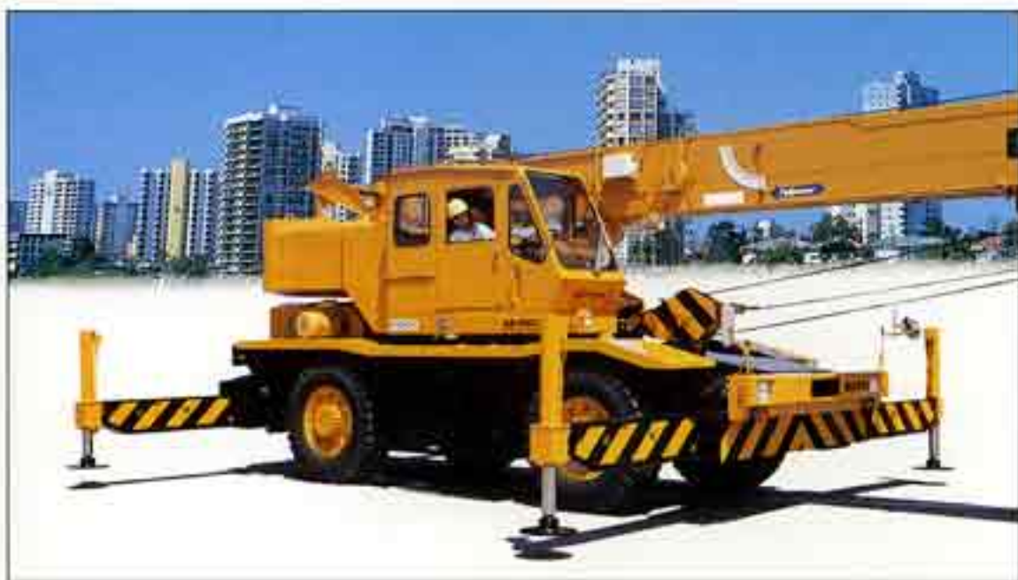
Outriggers can be controllable from operator's cab.
