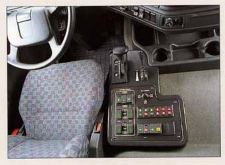
Independent rear steering with automatic locking system, hydraulic suspension control mounted at the side of the driver's seat.
