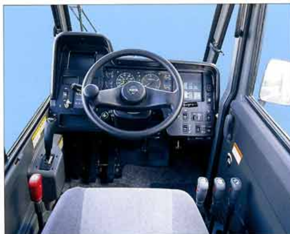
● Panel with shift position indicator
