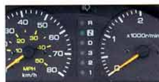
● Panel with shift position indicator
