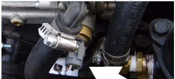
**6.** Remove the retainer clip for the LPG fuel temperature sensor and remove the sensor from the regulator body.
